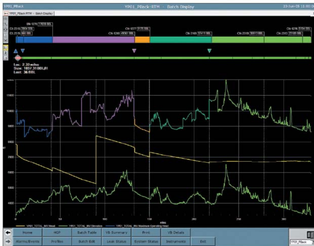
Figure 2. Batch tracking, leak detection and hydraulic gradient profile.
